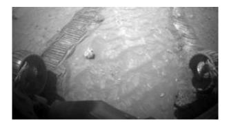
Spirit stopped short on its drive, apparently from the right front wheel encountering the partially buried rock visible next to that wheel. Image Credit: NASA/JPL-Caltech
