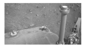
Engineering data from Spirit's power subsystem indicated that some dust blew off the rover's solar array on the following day, Sol 1812 (February 6, 2009). Image credit: NASA/JPL-Caltech
