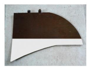
A prototype of an aerodynamic flap made of the new smart material. The smart material consists of thin plates containing carbon yarns that can carry a current, which heats and bends the material. Image credit: H. Drobez, et al.
