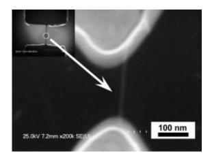
This is a black-and-white image of a micrograph from a scanning electron microscope of the electrodes (inset) and the single-walled carbon nanotube bridge structure. A colorized version of the micrograph of the electrodes was the cover photo for the Jan. 14 issue of Nanotechnology.
