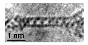
An electron microscope image of the smallest reported square-cross-section nanotube. Image courtesy Daniel Ugarte.
