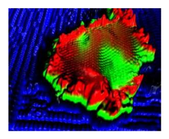
Atomic resolution scanning tunneling microscope image of a nanometer scale piece of graphene on silicon. Photo courtesy Joseph Lyding
