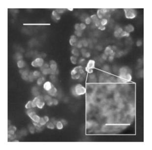
This is a microscopic view of silicon flakes designed to deliver drugs, then dissolve away. Credit: Luo Gu
