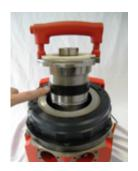
The adapter, here being inserted into the spindle (below), contains an RFID chip. The finger is pointing towards the coils which wirelessly transmit the information stored on the chip to the spindle. © Fraunhofer IMS
