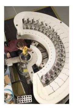
Top view of the MACS multiaxis detector system (seen before being enclosed in shielding material). With more neutrons striking the sample and more detectors surrounding it, MACS will greatly extend the capabilities of neutron inelastic scattering as a materials probe technique in nanotechnology and basic science. Principal investigator Collin Broholm of the Johns Hopkins University is seen examining the alignment of one of the 20 detection channels. Copyright: Robert Rathe
