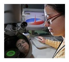
Argonne materials scientist Mihaela Tanase observes a small magnetic disk with a transmission electron microscope. Tanase discovered a new method to control the way the atoms in the magnetic disk orient themselves to form "nanoscale vortices," which are illustrated on the computer screen.
