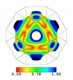
This is the Fermi surface of copper metal. The colors represent the curvature of the surface, which determines the propagation properties for electron waves. Credit: Martin Luther University Halle
