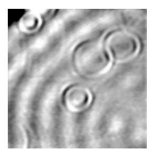
A scanning tunneling microscope recognizes spherical patterns on a copper surface (image section approx. nine times nine nanometers). These irregularities in electron distribution are caused by cobalt atoms deep inside the copper. Credit: Forschungszentrum Jülich
