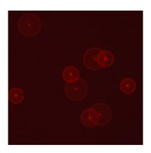
Fluorescence microscopy image of 100nm microspheres used to develop the DAC microscopy method for measuring molecules. Image: CSIRO
