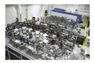
A "pathfinder" backplane is currently in production. It's used as a test to dry-run many of the critical, high-risk activities that are associated with the assembly, integration and test of the flight hardware. This photo emphasizes the assembly tools (silver-colored) which keep all the backplane (black tubes) in place as they are bonded. Credit: Northrop Grumman
