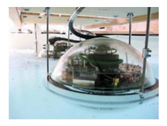
Two digital optical modules (DOMs) freeze into place in an IceTop tank on the surface of Antarctica. The IceTop array is a part of the IceCube Neutrino Observatory, an enormous telescope that is using high-energy neutrinos and cosmic rays to learn about distant cosmological events like supernovas and gamma-ray bursts. Photo: Tom Gaisser
