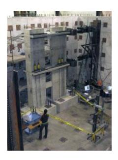
Engineers constructed a four-story, 40-percent replica of a building in a laboratory to test their new technique for bracing high rise buildings in earthquake zones. They simulated an earthquake by pushing and pulling the building with hydraulics. Image: Remy Lequesne
