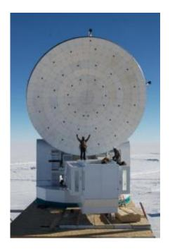
The South Pole Telescope takes advantage of the clear, dry skies at the National Science Foundation's South Pole Station to study the cosmic background radiation, the afterglow of the big bang. The SPT measures eight meters (26.4 feet) in diameter. Photo by Jeff McMahon
