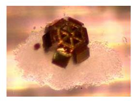
This optical microscopy image show a tetherless microgripper holding on to a piece of bovine bladder tissue retrieved from a tissue sample placed at the end of a narrow glass capillary tube.
