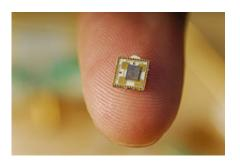
This 60 GHz single-chip CMOS radio-frequency device, developed at the Georgia Electronic Design Center by Joy Laskar and Stephane Pinel, is currently the world's most integrated chip for 60 GHz wireless applications.
