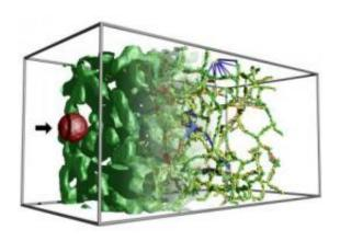
After using the algorithm to determine the filament structure of an aerogel -- a lightweight foam used in shielding electronic equipment in satellites -- the researchers were able to compute changes to its structural integrity by the simulated impact of a micrometeorite traveling at 10,000 miles per hour (red sphere on left). Image: Attila Gyulassy/UC Davis Copyright UC Regents
