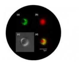
Pictured are micrographs of microcapsule syringes. a) Blue laser light shows lithographic microcapsule shell in green. Hole in the encapsulation can be seen as discontinuous circle. b) Green laser light shows the red dye loaded into the microcapsule. c) Differential Interference Contrast microscope image of microcapsule. d) Overlay of a) and b) showing image of filled capsule. Credit: Darrell Velegol, Penn State
