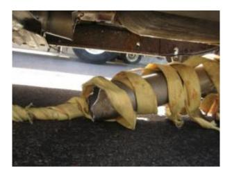
Here, the Department of Homeland Security S&T's Safe Quick Undercarriage Immobilization Device (SQUID) is entangled in the undercarriage of a vehicle. Credit: DHS S&T
