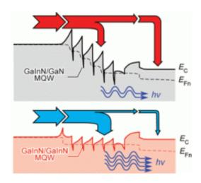
Band diagram of conventional GaInN/GaN active region and new polarization-matched GaInN/GaInN active region of a light-emitting diode.
