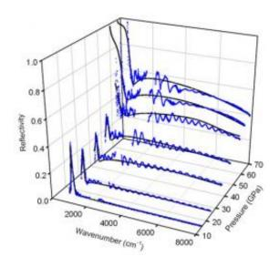
Room-temperature infrared reflectivity spectra of SiH4 at selected pressures up to 67.2 GPa. The blue squares are the measurement results. The solid lines represent model fits to the data. The small gap in the spectrum near 2000 cm-1 is due to diamond anvil absorption.
