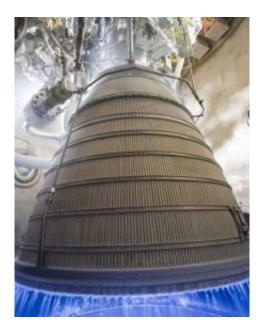
The Common Extensible Cryogenic Engine, or CECE, is fueled by a mixture of liquid oxygen and liquid hydrogen chilled to sub-zero temperatures. Image Credit: Pratt & Whitney Rocketdyne
