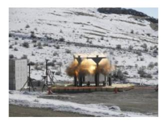
A full-scale separation test of the forward skirt extension for the Ares I-X flight test at its facility in Promontory, Utah on January 29, 2009. (Image: NASA/ATK)
