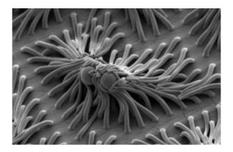
Illustration of the adhesive and particle trapping potential of the helically assembling bristle. Shown: Low-magnification SEM showing the capture of the 2.5-mm polystyrene spheres. Scale bar, 10 mm. Courtesy of Aizenberg lab at the Harvard School of Engineering and Applied Sciences
