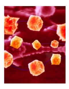
This image, taken with a scanning electron microscope and digitally colorized and enhanced, shows a new precise biosensor for detecting blood glucose and other biological molecules using hollow structures called single-wall carbon nanotubes anchored to gold-coated "nanocubes." The device resembles a tiny cube-shaped tetherball anchored to electronic circuitry by a nanotube about 25,000 times thinner than a human hair. (Jeff Goecker, Discovery Park, Purdue University)
