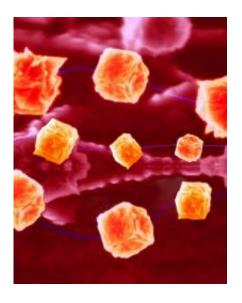
This image, taken with a scanning electron microscope and digitally colorized and enhanced, shows a new precise biosensor for detecting blood glucose and other biological molecules using hollow structures called single-wall carbon nanotubes anchored to gold-coated "nanocubes." The device resembles a tiny cube-shaped tetherball anchored to electronic circuitry by a nanotube about 25,000 times thinner than a human hair. (Jeff Goecker, Discovery Park, Purdue University)
