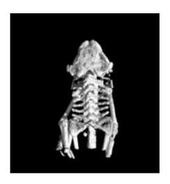
The tomographic image of the frog above was reconstructed from 60 transmission projections recorded over 360 degrees. The reconstructed data set has 192 x 192 x 240 voxels, and an isotropic pixel size of 80 microns cubed. A standard filtered back projection algorithm with a Hamming cut off was used. Credit: Prof. Franz Pfeiffer and Lyncean Technologies
