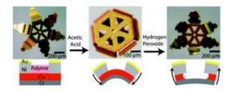
Engineers have developed tiny, robotic hands -- also known as microgrippers -- that could be used in lab-on-a-chip applications. Credit: American Chemical Society
