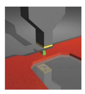
Rendering of the key elements of a magnetic resonance force microscope. An ultrasensitive silicon cantilever detects the tiny magnetic force between a nanoscale magnetic tip (green) and the hydrogen nuclei present in the virus particles placed at the end of the cantilever (blue, seen in the reflection). Nanoscale magnetic resonance imaging is achieved by manipulating the hydrogen nuclei in the sample with a radiofrequency magnetic field generated by
