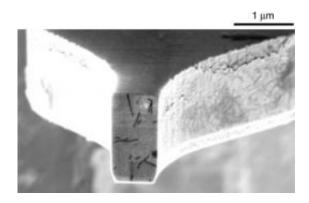
Electron micrograph showing the end of the silicon cantilever with several virus particles attached. Adapted from Fig. 1 of the PNAS article.
