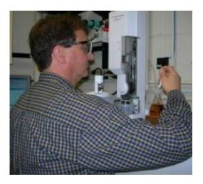
NIST chemist Tom Bruno demonstrates sampling of biodiesel fuel for injection into a gas chromatograph-mass spectrometer, an instrument that separates and identifies the components of a mixture. Credit: Ost, NIST
