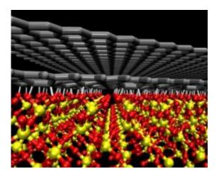
Researchers at Rensselaer have developed a new method for controlling the conductive nature of graphene. Pictured is a rendering of two sheets of graphene, each with the thickness of just a single carbon atom, resting on top of a silicon dioxide substrate. Credit: Rensselaer/Shemella
