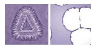
Crystallization (left) occurs as polymers harden into thin films, which are used widely in electronics technology. But when dewetting (right) also occurs, inhomogeneities in the film can degrade performance. NIST scientists found that temperature determines which process dominates film formation, and that keeping certain angles between crystallization fronts can largely prevent dewetting. Image: NIST
