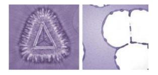
Crystallization (left) occurs as polymers harden into thin films, which are used widely in electronics technology. But when dewetting (right) also occurs, inhomogeneities in the film can degrade performance. NIST scientists found that temperature determines which process dominates film formation, and that keeping certain angles between crystallization fronts can largely prevent dewetting. Image: NIST
