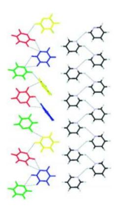
This is a diagram of the crystal structure of deuterated pyridine. (c) Wiley-VCH 2008
