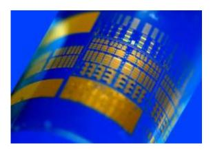
This example of a curved photodetector array was developed by University of Wisconsin-Madison Electrical and Computer Engineering Associate Professor Zhenqiang (Jack) Ma and colleagues. Inspired by the human eye, Ma's curved photodetector made of flexible germanium could eliminate the photo distortion that occurs in conventional photo lenses. Photo courtesy Zhenqiang Ma
