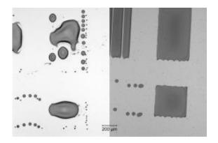
In order for printed electron devices to work, the researchers need to match the properties of the ink and the substrate surface to one another. The untreated insulator (left) is difficult to wet, unlike the surface-treated insulator (right). © Fraunhofer IISB
