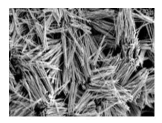
This is a pile of nanowires before assembly. Credit: Penn State
