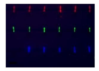
These nanowires, tagged with DNA are assembled, and have been exposed to complementary DNA that is tagged with fluorescent dyes. The complementary DNA attached to the nanowires showing that the wires assembled in the proper locations. Credit: Penn State
