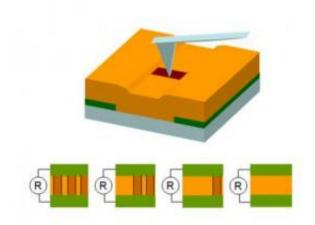
Scanning probe tips can be used to control the number and arrangement of conducting domain walls in bismuth ferrite (gold) between electrodes (green), thus creating useful devices on the nanoscale. For example, current can be incrementally controlled by creating or erasing domain walls, as at bottom. Credit: Lawrence Berkeley National Laboratory, UC Berkeley
