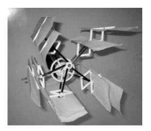
A prototype design of the cyclogyro craft with five pantograph-based variable wing
