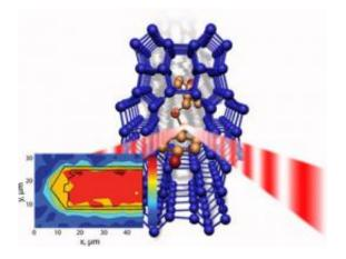
Molecules formed during a catalytic reaction in the zeolite micropores are identified using synchrotron infrared light.
