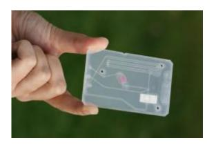
This card is part of a system hoping to diagnose malaria far from any laboratory. The red circle at the center contains dehydrated antibodies that can be stored for months without refrigeration. The lines are tiny channels that guide a blood sample through the card, and the blood mixes with various solutions for set periods of time. When the fluids reach the white rectangle, a red spot will appear, and its intensity shows whether the patient is infected. Photo: Dean Stevens
