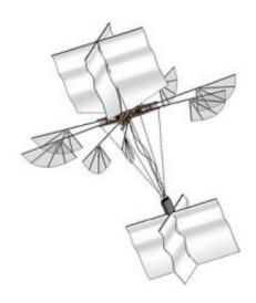
Four sets of small flapping wings and stabilizing sails give the vehicle the ability to right itself from any position, something even helicopters can't do.
