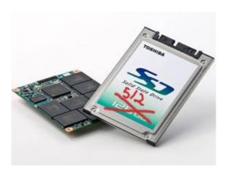
(PhysOrg.com) -- Toshiba announced today the expansion of their line up of NAND-flash-based solid state drives (SSD) with the industry's first 2.5-inch 512 GB SSD and a broad family of fast read/write SSD's based on 43 nanometer Multi-Level Cell NAND.
