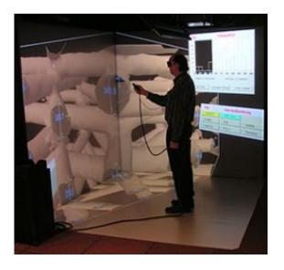
Researcher Bill George is in the immersive environment with the corrected location and orientation measurements, measuring an enlarged version of the engineered lattice structure that is about 2 to 3 millimeters. NIST-developed software greatly increased the accuracy of the immersive environment by correcting the tracking of the location and orientation of the sensors attached to the 3-D glasses and the wand that George holds in his hands. Credit: NIST
