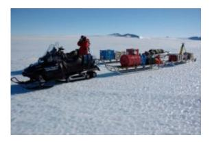
Taking a tea break out on the blue ice. The sledges are loaded with petrol, camping gear, a survival kit, food and of course scientific equipment. All trips out are being used to survey the height of the ice surface using kinematic GPS. The Global Navigation Satellite System (GNSS) antenna mounted on the tripod is on the back of the sledge. The picture shows a blue ice area without snow cover.
