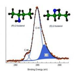
1s XPS spectrum of (R)-2-butanol adsorbed on permalloy at 90 K obtained at the start of a photolysis series. The points are the raw data; the dashed lines are the individual fitted components, and the solid line is the synthesized curve. The filled in region represents the C-O peak, which directly probes the chiral carbon. Also shown are models of (S)- and (R)-2-butanol. Image: ANL
