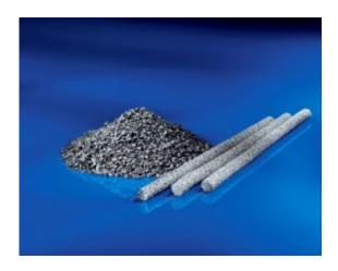
A plastic-metal hybrid as a granulate or a strand. In the next step the conductive material can be plasticized (softened) again and applied as a printed circuit board. © Fraunhofer IFAM
