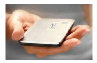
(PhysOrg.com) -- The Novatel MiFi portable broadband hotspot card does the job of a 3G modem and wireless router combined. The MiFi can connect to either an EVDO Rev. A or HSPA signal. The connection is then shared via a WiFi connection.
