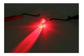
This carbon-nanotube coated smart yarn can conduct enough electricity from a battery to power a light-emitting diode device. Researchers can use its conductivity to design garments that detect blood.
