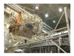
The Lunar Reconnaissance Orbiter entering the Thermal Vacuum Chamber at NASA's Goddard Space Flight Center in Greenbelt, Md. Credit: NASA's Goddard Space Flight Center
